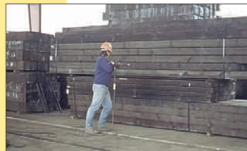
Core samples are removed by a hollow drill bit called an increment borer.
