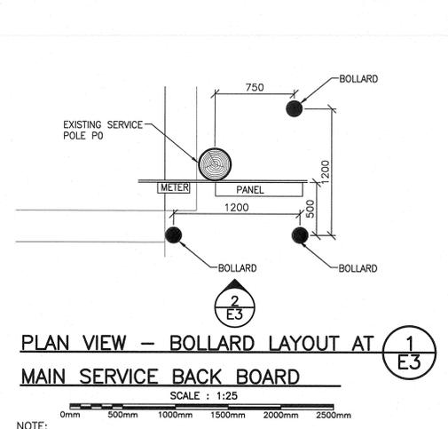
**PLAN VIEW - BOLLARD LAYOUT AT MAIN SERVICE BACK BOARD**
