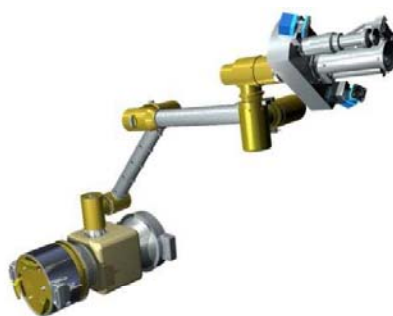
FIGURE 1-5: CONCEPT OF SMALL DEXTEROUS ROBOTIC SYSTEM
