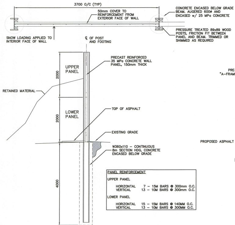
**PRECAST CONCRETE PANEL FENCING DETAIL**
