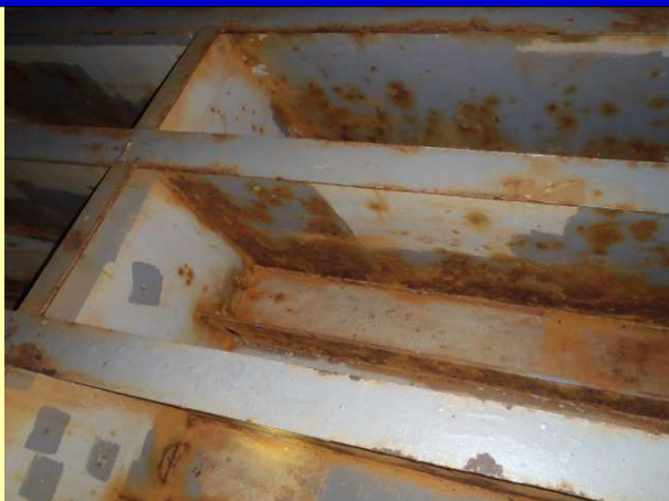
Bilge areas are in poor condition
