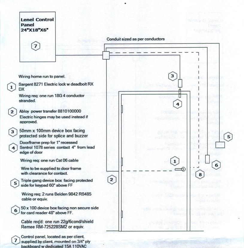
Alternate wiring replacing note 2 if electric strike is used instead of electric mortise lock.
