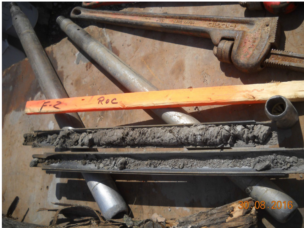
Picture 4 : Slotted spoon sampling - Drilling F-2
