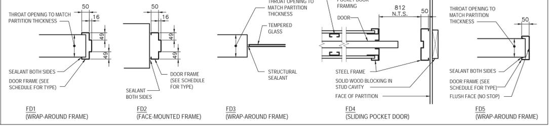
**DOOR AND FRAME ELEVATIONS, DOOR FRAME DETAILS**
