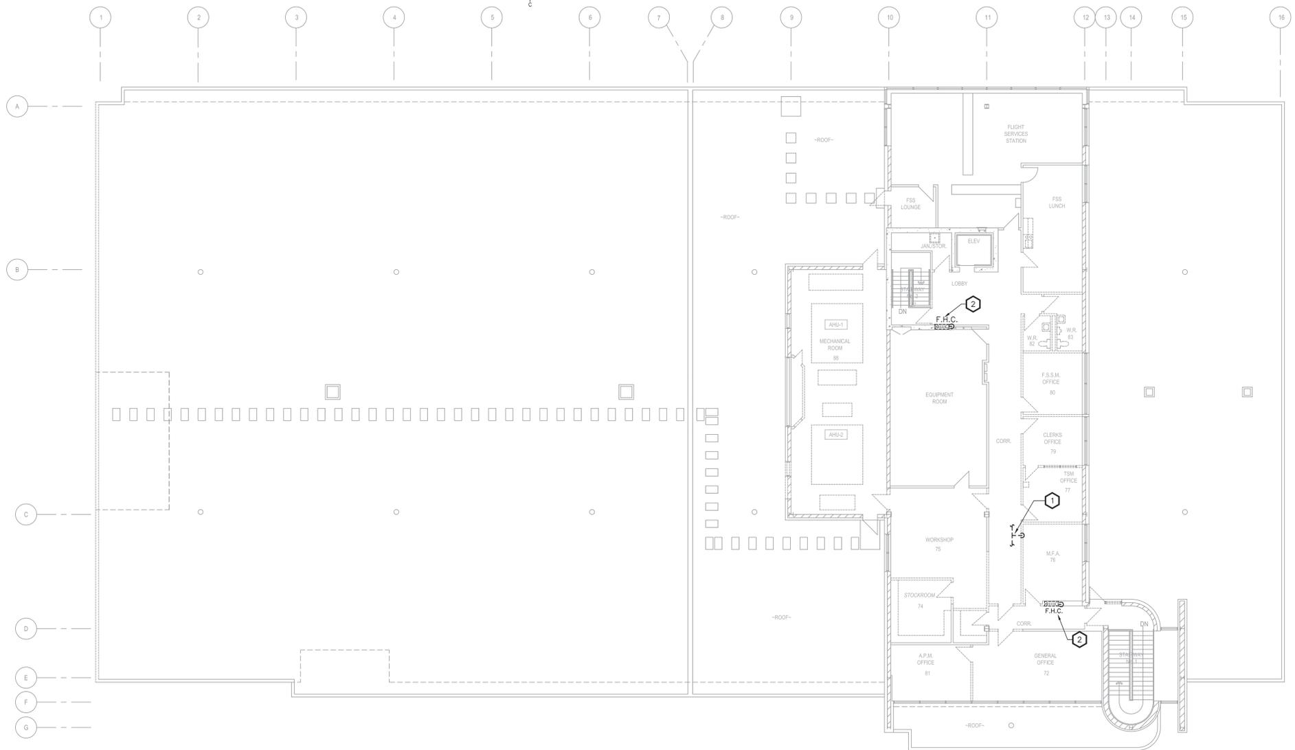
FLOOR PLAN - FIRE PROTECTION DEMOLITION, LEVEL 2
