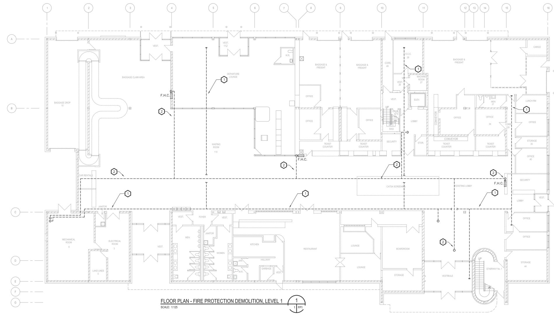
**FLOOR PLAN - FIRE PROTECTION DEMOLITION, LEVEL 1**
