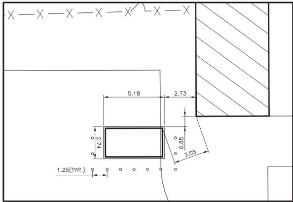
**DIESEL STORAGE TANK CONCRETE PAD LOCATION**
