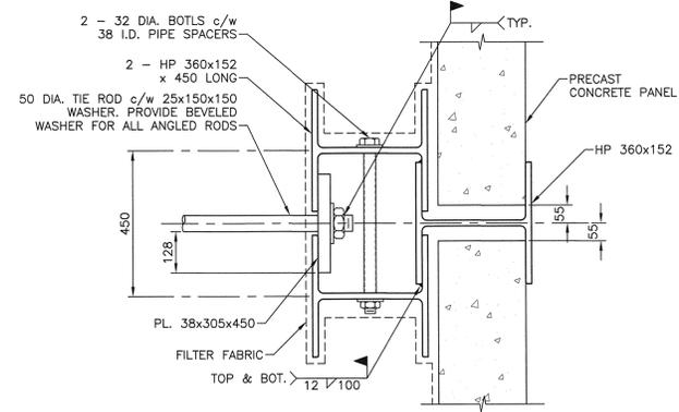
**DETAIL - TIE-ROD CONNECTION TO H-PILE**
