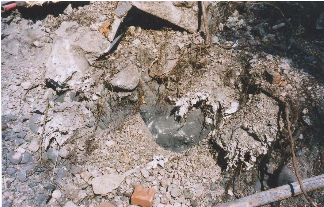
Photograph No. 2: Air cell insulation embedded in contaminated soil at northeast corner of Fog Alarm Building.
