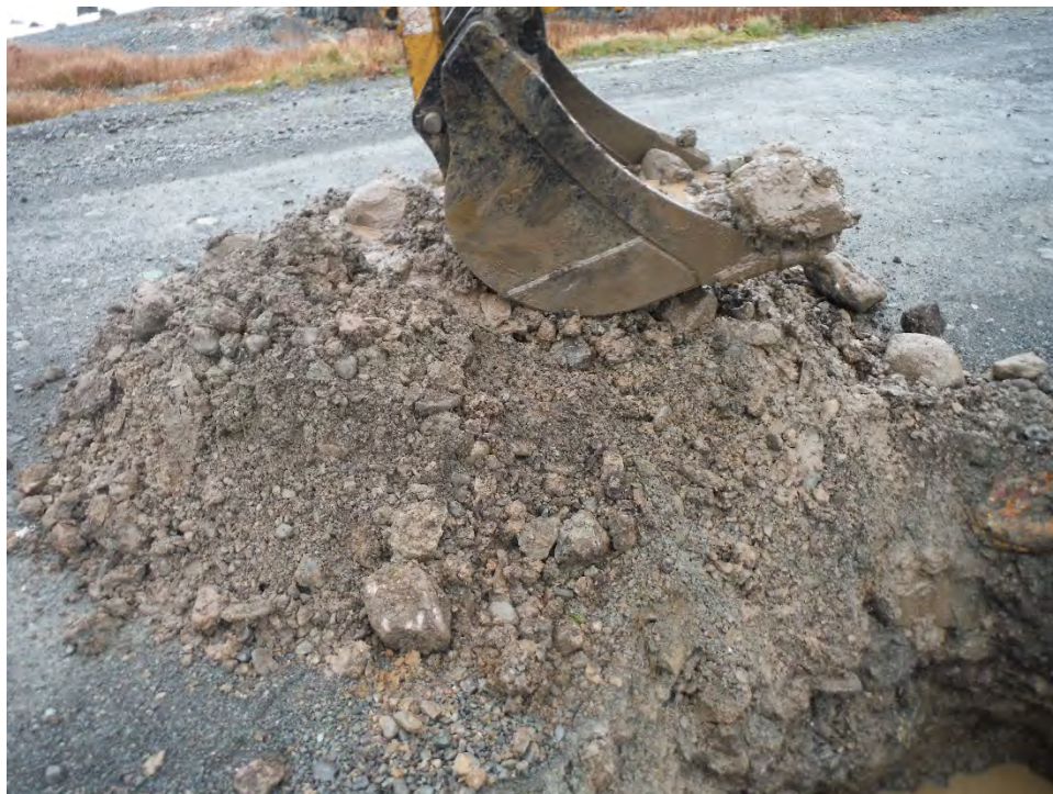
Test Pit TP-27 Spoil Pile
