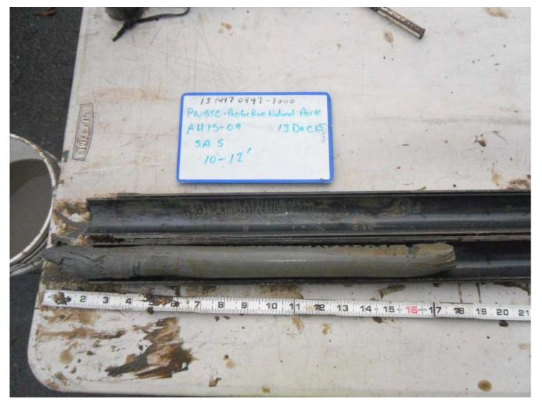
Photograph 16: Example of silty clay material in a split spoon from AH15-09 at Washroom #4 located in the south portion of Green Point Campground
