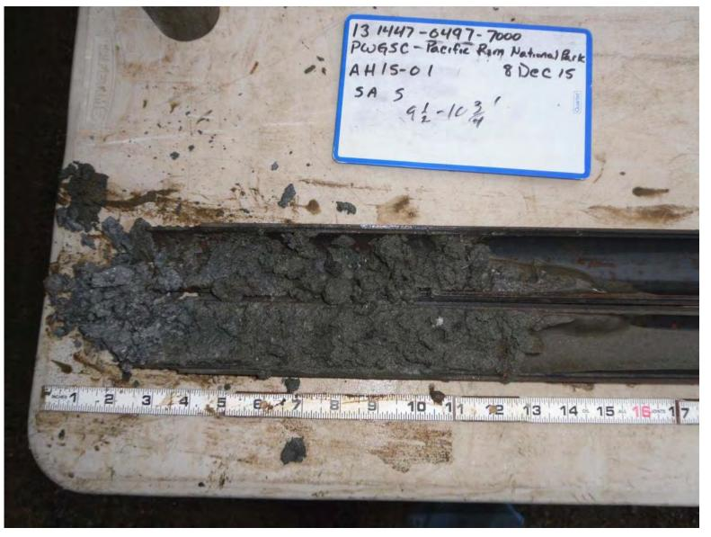
Photograph 8: Example of sand with silt and gravel material in a split spoon from AH15-01 at the Incinerator Rock washroom
