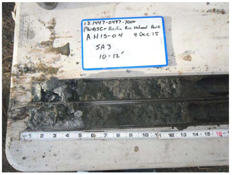
Photograph 10: Example of compact to dense sand with silt and gravel material in a split spoon from AH15-04 at the Long Beach north washroom
