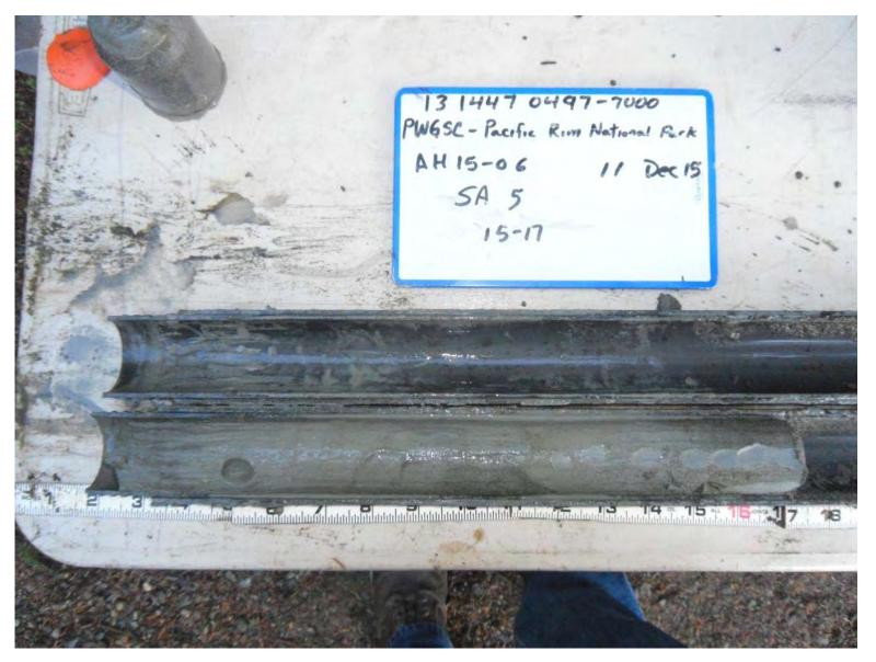
Photograph 11: Example of silty clay material in a split spoon from AH15-06 at the Long Beach south washroom
