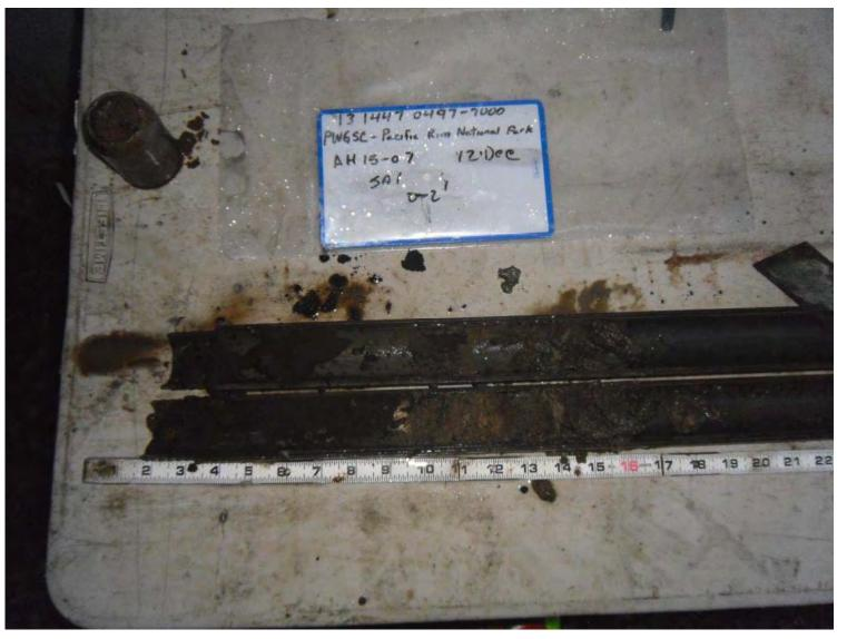
Photograph 12: Example of surficial sand material in a split spoon from AH15-07 at Washroom #1 located in the north portion of Green Point Campground
