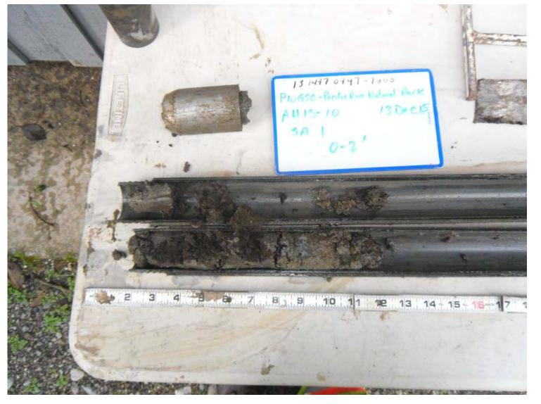
Photograph 15: Example of clayey silt and sand material in a split spoon from AH15-10 at Washroom #4 located in the south portion of Green Point Campground
