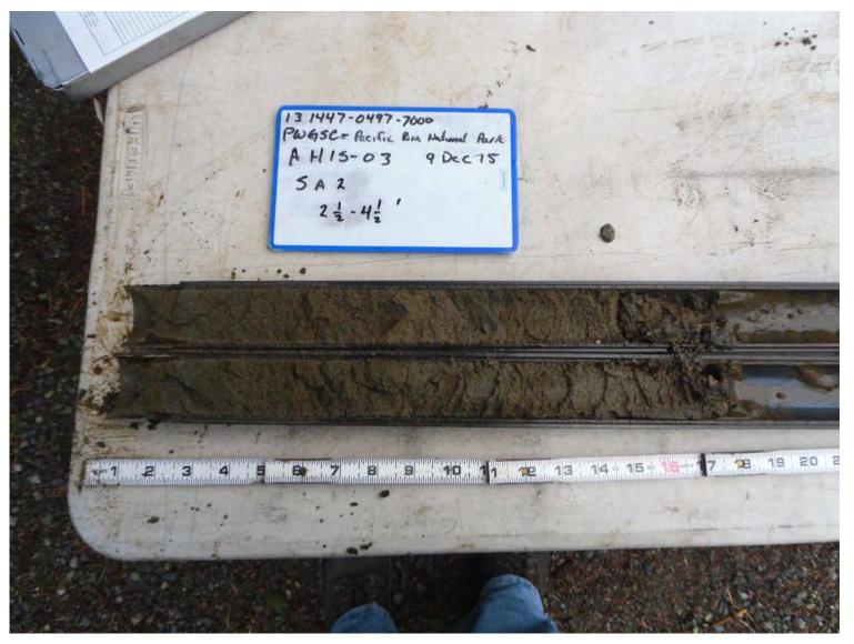
Photograph 9: Example of compact to dense sand with silt and gravel material in a split spoon from AH15-03 at the Long Beach north washroom
