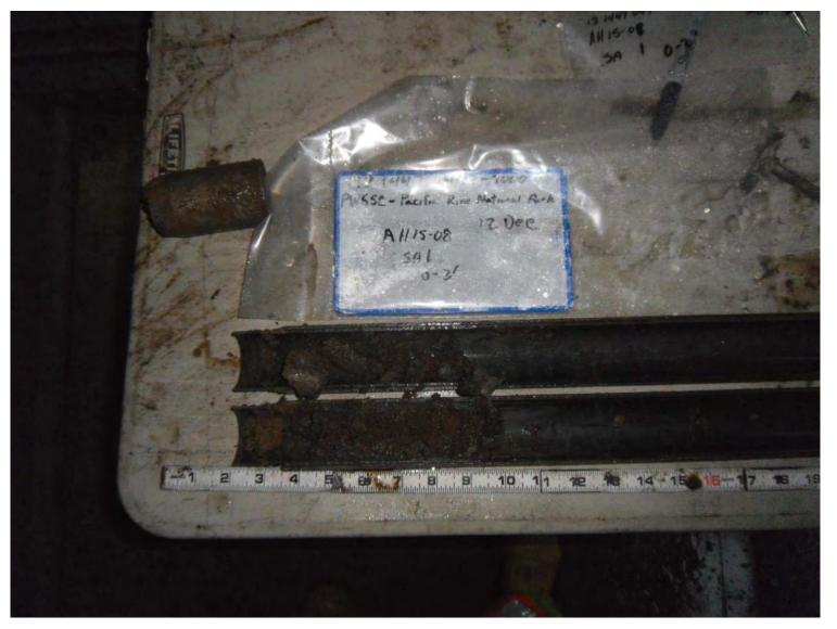
Photograph 14: Example of surficial sand material in split spoon from AH15-08 at Washroom #1 located in the north portion of Green Point Campground
