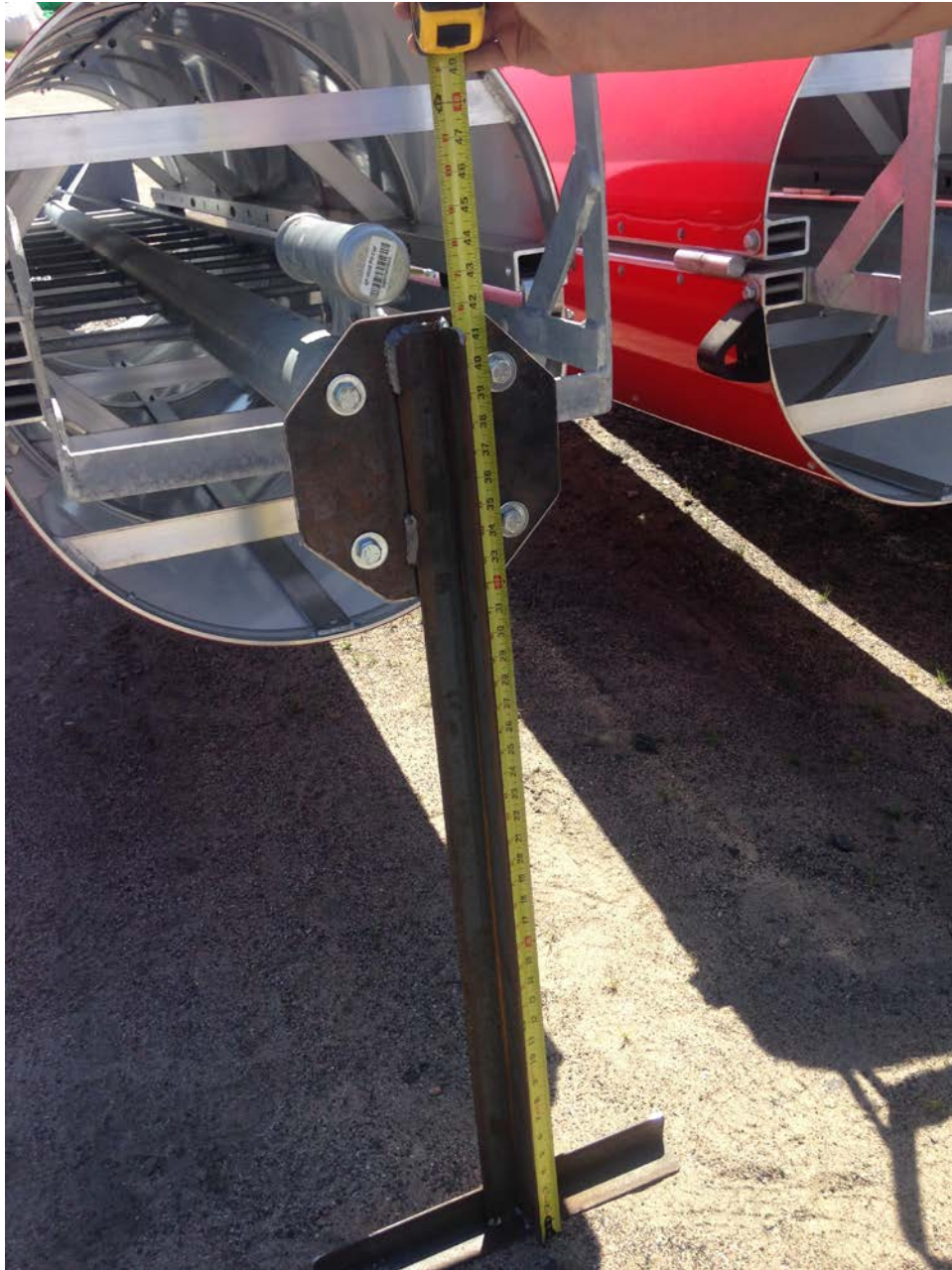
Figure 5: Typical strut connected to the top point of 16' pipemast navaid for transportation (strut supplied by CCG)
