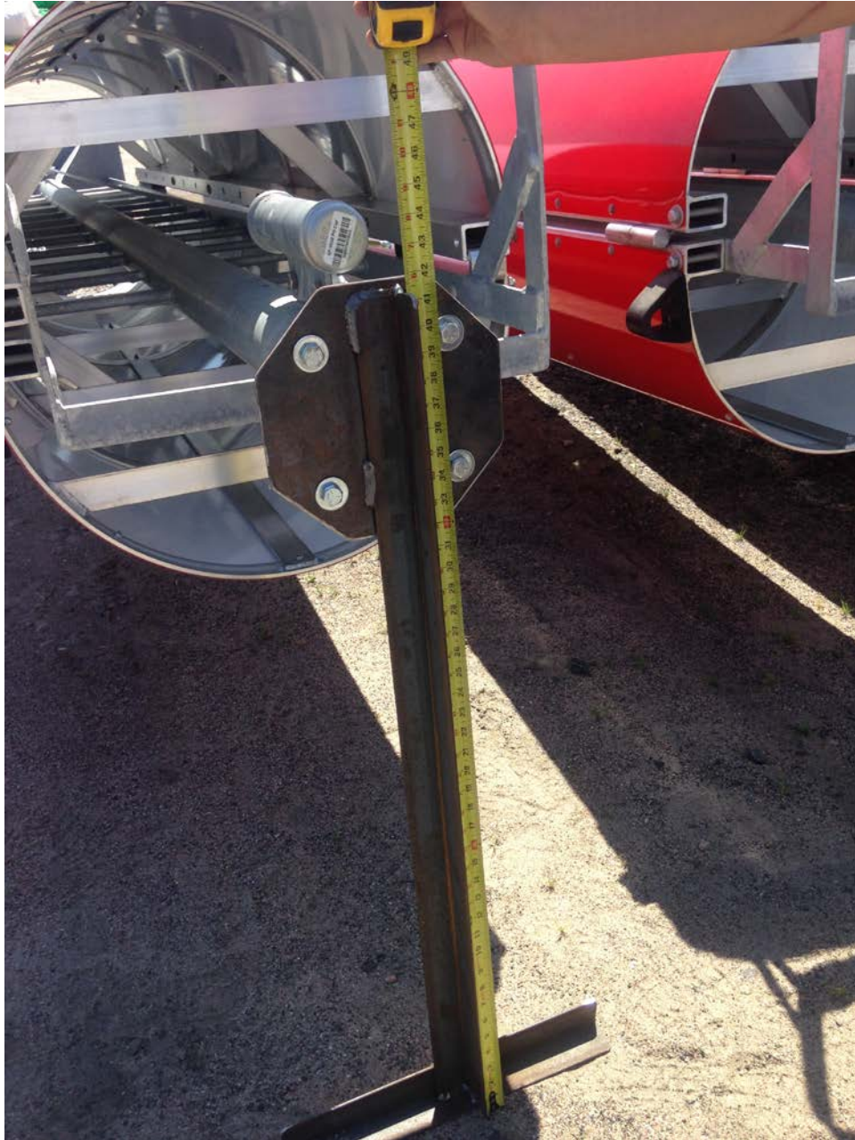
Figure 19: Typical strut connected to the top point of 16' pipemast navaid for transporation (strut supplied by CCG)
