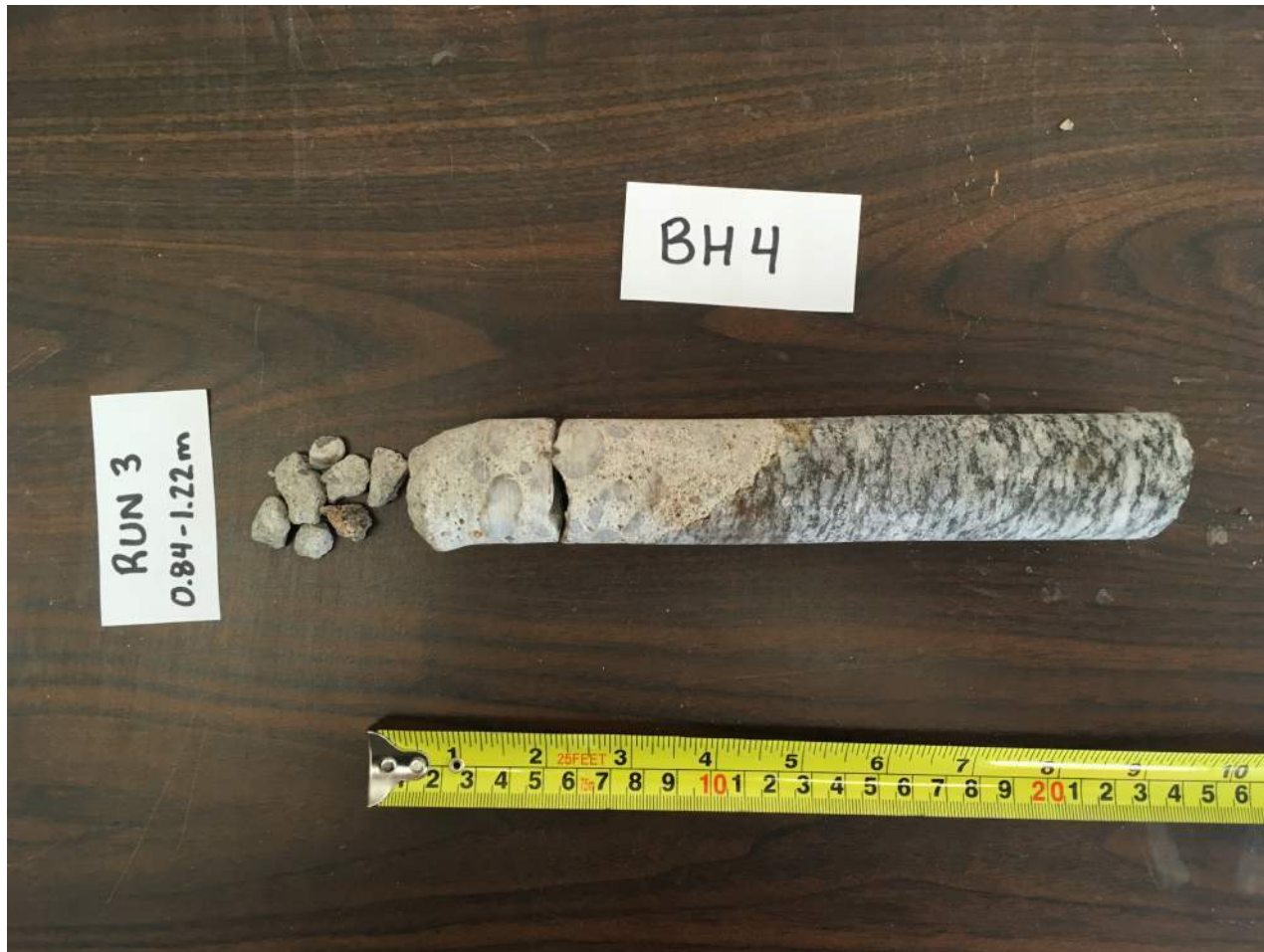
BOREHOLE 4 Run 3 Depth: 0.84 to 1.22m
