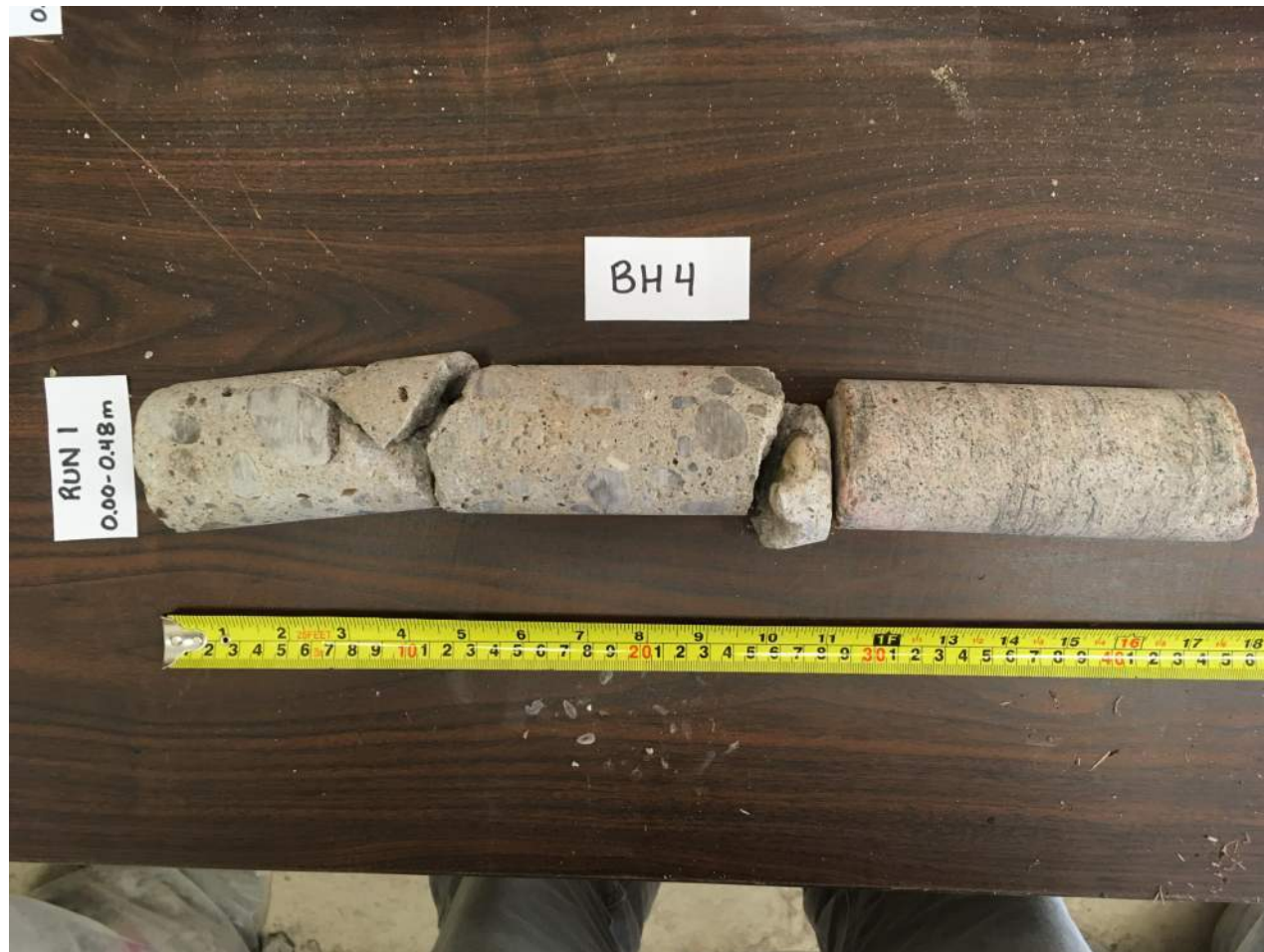
BOREHOLE 4 Run 1 Depth: 0.0 to 0.48m
