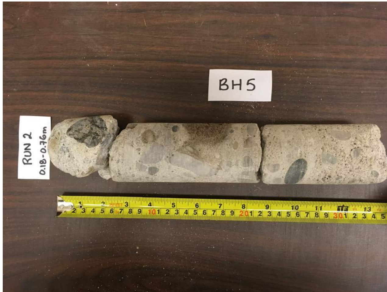
BOREHOLE 5 Run 2 Depth: 0.18 to 0.76m
