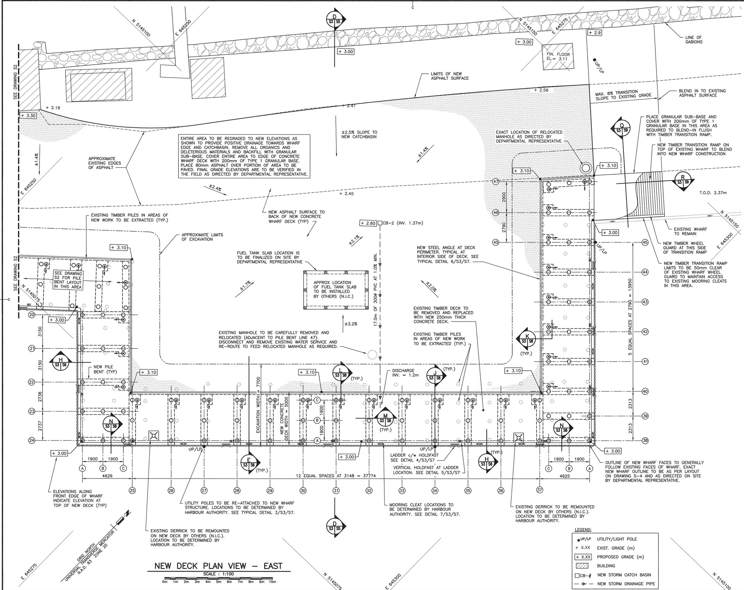
ENTIRE AREA TO BE REGRADED TO NEW ELEVATIONS AS SHOWN TO PROVIDE POSITIVE DRAINAGE TOWARDS WHARF EDGE AND CATCHBASIN. REMOVE ALL ORGANICS AND DELETERIOUS MATERIALS AND BACKFILL WITH GRANULAR SUB-BASE. COVER ENTIRE AREA TO EDGE OF CONCRETE WHARF DECK WITH 200mm OF TYPE 1 GRANULAR BASE. PLACE 80mm ASPHALT OVER PORTION OF AREA TO BE PAVED. FINAL GRADE ELEVATIONS ARE TO BE VERIFIED IN THE FIELD AS DIRECTED BY DEPARTMENTAL REPRESENTATIVE.
