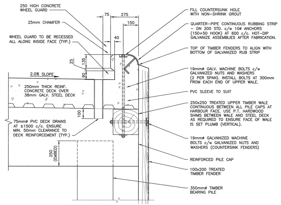
**TYPICAL WHEEL GUARD AND UPPER TIMBER WALE SECTION**
