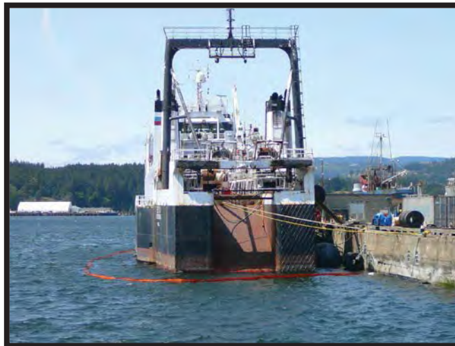
Containment boom around vessel during fuelling operations
