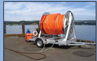
The EGD boom reel and containment boom
