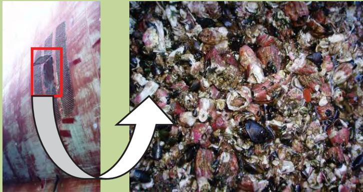
Sea chests such as this one from a cruise ship docked at the EGD often contain a significant amount of marine life. If not managed appropriately this marine life has the potential to negatively impact the local ecosystem of the harbour
