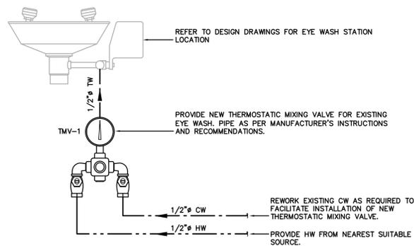
**3 DETAIL -EYE WASH THERMOSTATIC MIXING VALVE**
