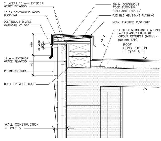
ROOF EDGE AT EXISTING ITS STORAGE BUILDING (HIGH SIDE) (6 A10)
