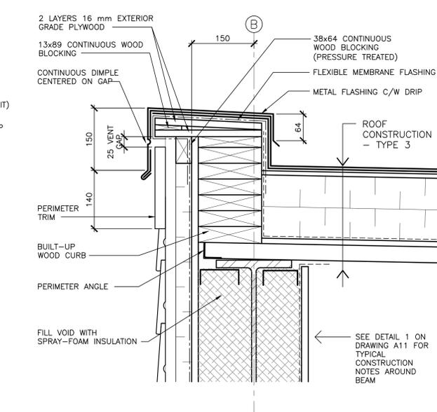
ROOF EDGE AT ITS STORAGE BUILDING EXTENSION (HIGH SIDE) (8 A6, A10)
