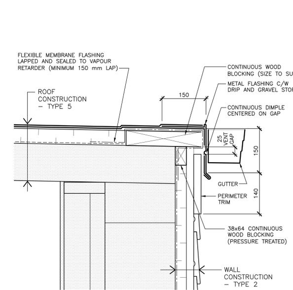
ROOF EDGE AT EXISTING ITS STORAGE BUILDING (LOW SIDE) (7 A6)
