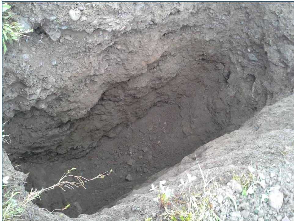
Photo 20: Lithology observed in TP16-1 – the surface unit consisting of a brown sand with some gravel, pebbles, and cobbles throughout is visible at the top portion of the photograph
