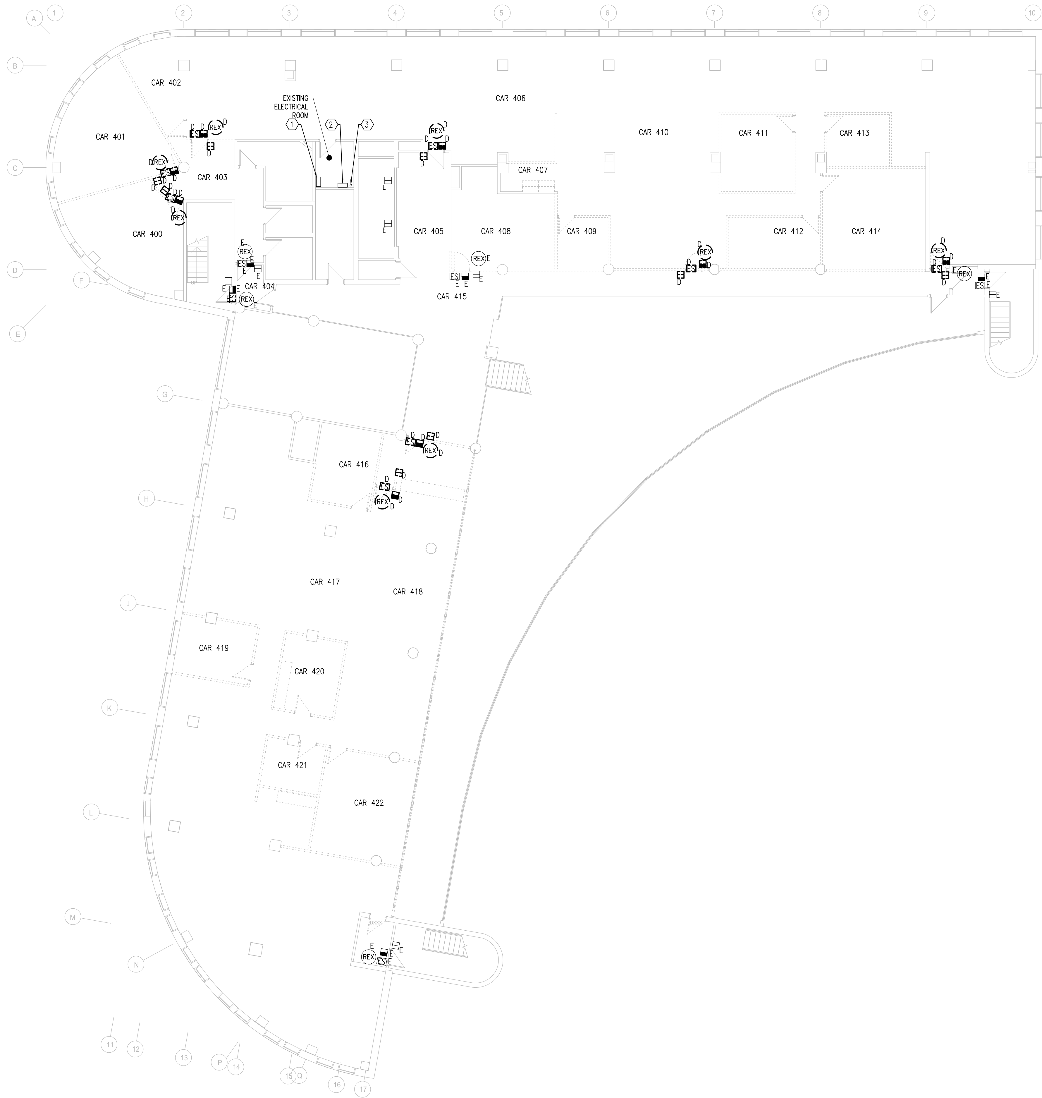
1 EXISTING/DEMOLITION ACCESS CONTROL SYSTEMS LAYOUT T1.2 1:125
