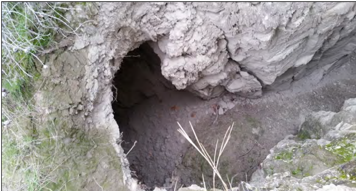
Photograph 8: View looking down into sinkhole at top of steep bluff where water has emerged from sub-surface flow.
