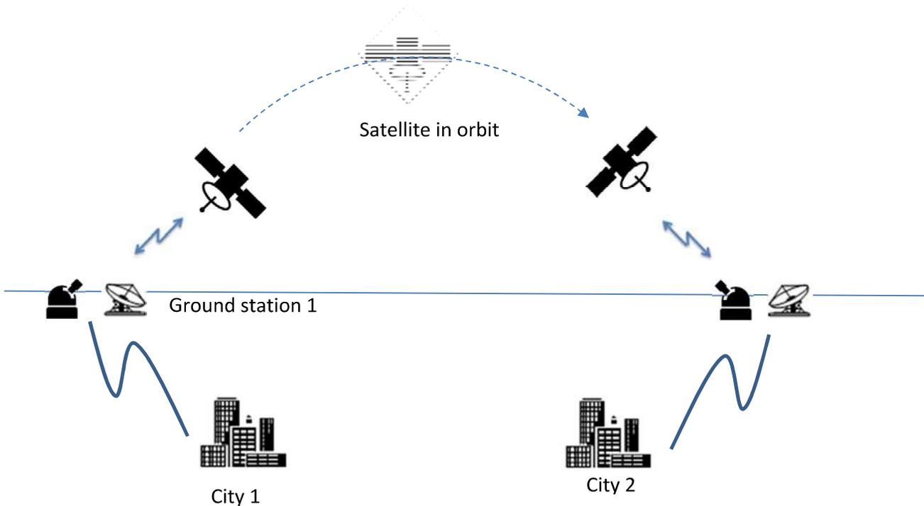
The proposed system is based on a quantum photon uplink from ground to a satellite. The quantum source is located at the ground station and the quantum receiver (photon polarization detectors) is located on the satellite.
