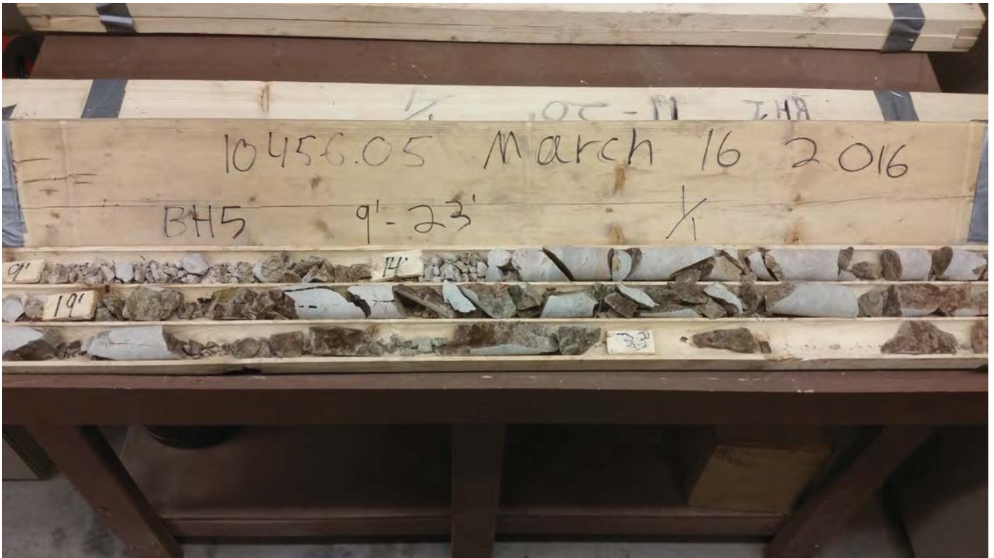
PHOTO 3 - Slate bedrock cores from BH5 (2.74 to 7.0 metres)
