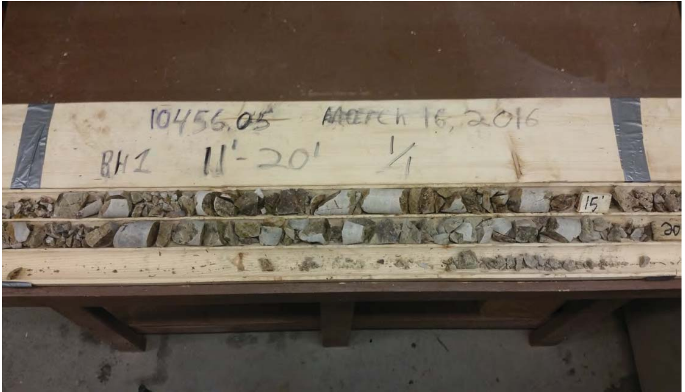
PHOTO 1 - Slate bedrock cores from BH1 (3.3 to 6.06 metres)
