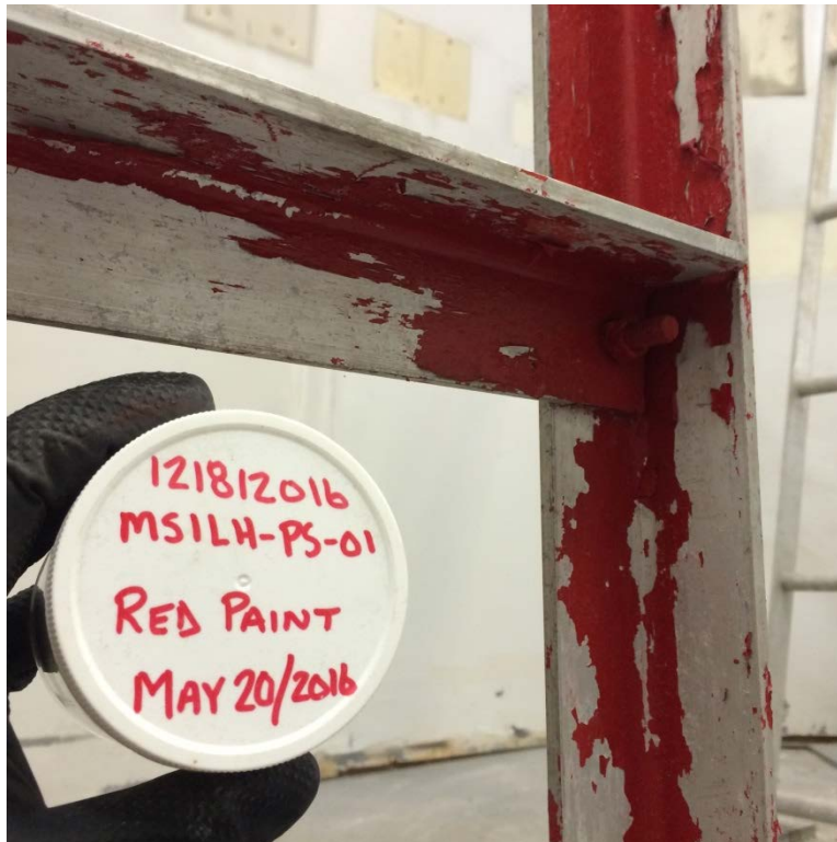
PHOTO 12: View of red paint on metal on Level 2. Samples of red paint chips collected from ladders on this level and other levels were combined into sample PS-01 which was found to be lead leachate toxic (i.e. lead leachate concentration was \geq 5 mg/L).
