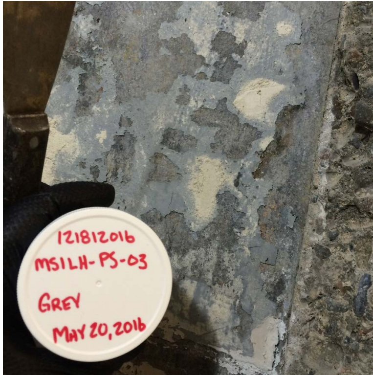
PHOTO 13: View of grey floor paint from Level 3. A sample of grey paint chips collected from this area (PS-03) was found not to be lead leachate toxic (i.e. lead leachate concentration was <5 mg/L).
