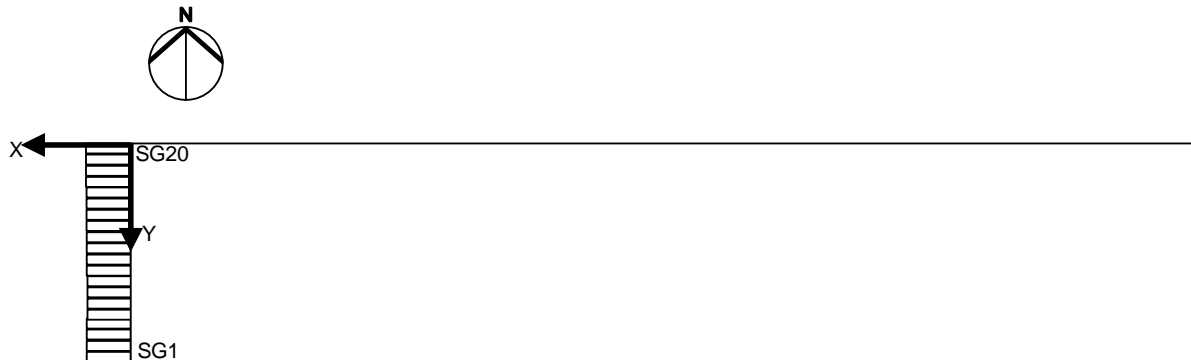
Figure 5-1: Coordinate system for the Segmented Wave Generator
