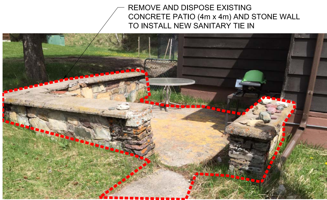
1 - DETAIL CONCRETE PATIO AND STONE WALL REMOVAL NTS
