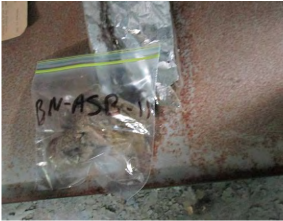
Photo 13: View of insulation with foil backing sample BN-ASB-11.
