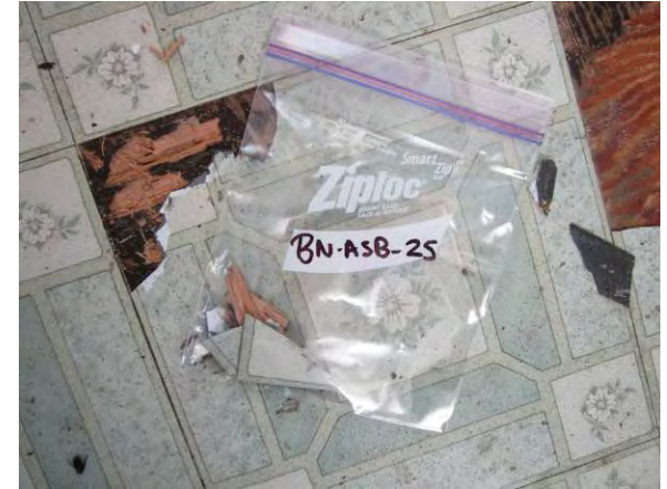
Photo 27: View of light green and beige vinyl floor tile with black mastic sample BN-ASB-25.
