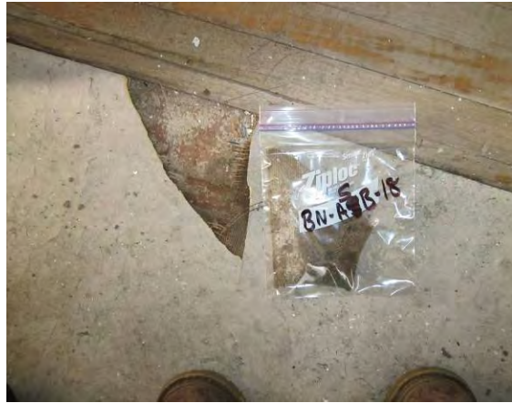
Photo 20: View of grey wood panel flooring with mesh backing and grey adhesive sample BN-ASB-18.
