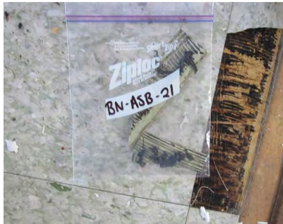
Photo 23: View of grey with green and white fleck vinyl floor tile sample BN-ASB-21.
