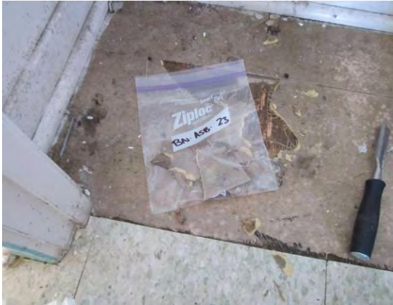
Photo 25: View of brown rolled flooring with mesh backing and adhesive sample BN-ASB-23.
