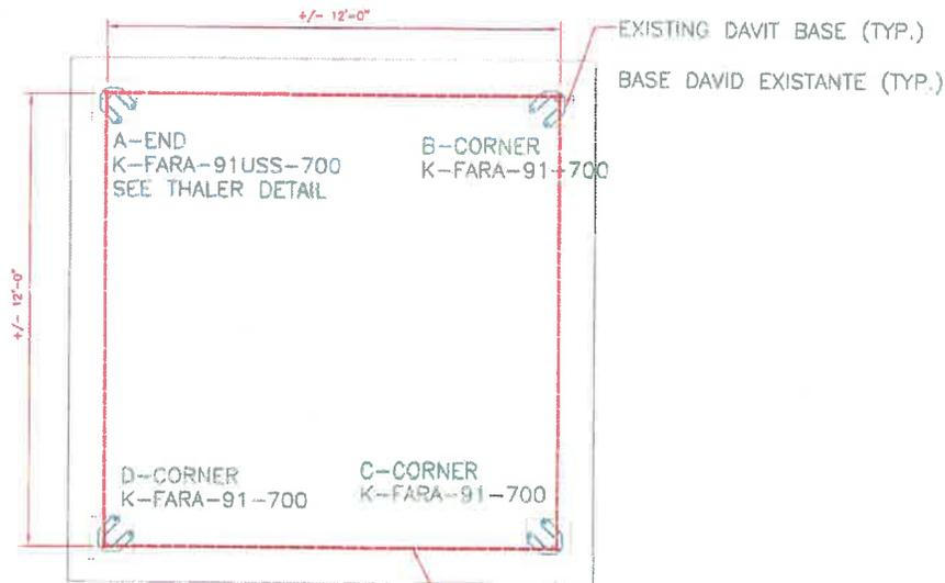
NEW CONTINUOUS FLEXIBLE HORIZONTAL LIFE-LINE K-700 (MAX 2 WORKER) BOLTED TO THE EXISTING DAVIT BASES. EXISTING OUTER SLOTS IN BASE SHALL BE USED FOR BOLTED CONNECTION.
