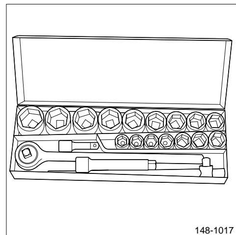
Figure 2 Socket wrench kit (including ratchet wrench, ratchet wrench extension and sockets).
