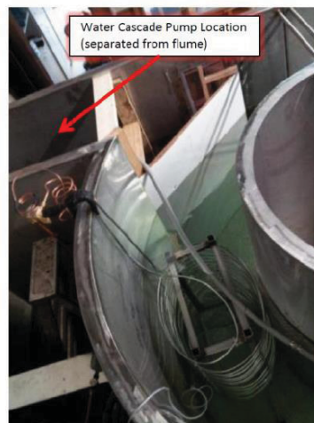
Water Chiller Heat Transfer Coil and Water Cascade Pump Location
