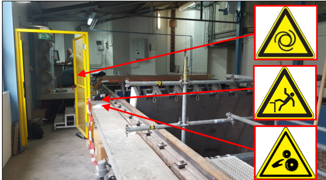
Figure 2-1: Safety symbols on entrance door
