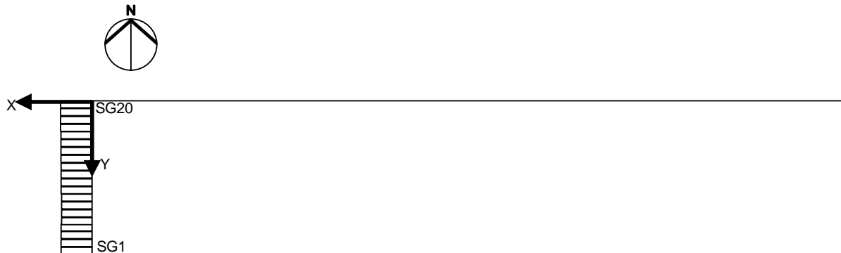
Figure 5-1: Coordinate system for the Segmented Wave Generator
