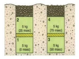
Per Fig. 1: 20 kg total weight of charge; 25 msecs delay between charges and blast holes and decking of charges within holes. (Fisheries and Oceans Canada, 2015)
