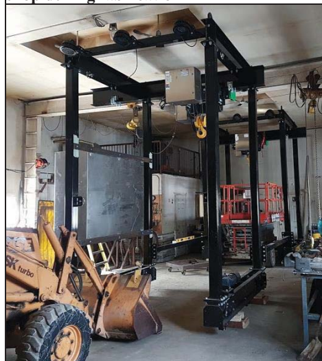
Figure 4 - Stoplog lifter on East Dam – in shop during fabrication
