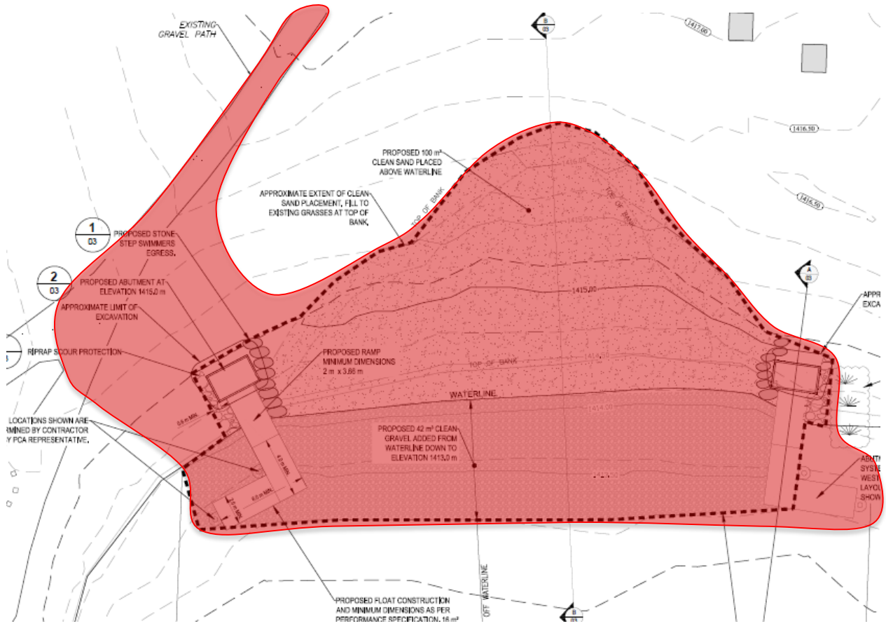
Figure 3. Proposed access and construction footprint/disturbance impact limitations for Area 1 (denoted by red area).
