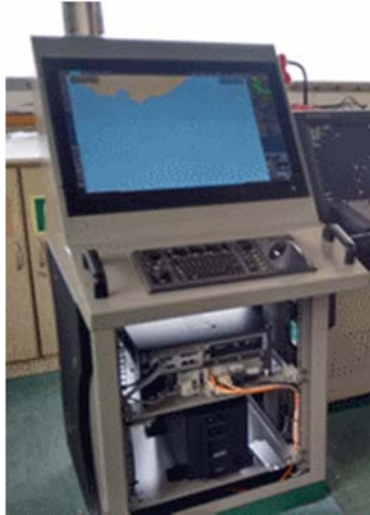
Figure 8: Port Ship Control Station and Bridgemaster Aft facing radar locations
