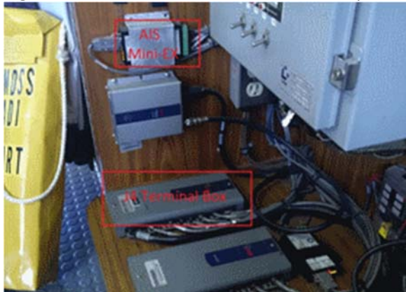
Figure 11: AIS J4 Terminal Box and Mini Expander
