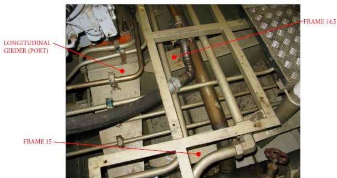
Figure 11: Main Engine Room- View of outboard (Port) engine support girder (looking aft)
