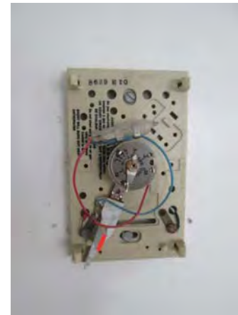
Photo 168: View of rectangular White-Rodgers thermostat (mercury-containing).
