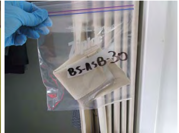
Photo 33: View of plastic/fabric-type material sample BS-ASB-30.
