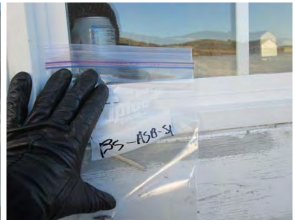
Photo 54: View of white window caulking sample BS-ASB-51.
