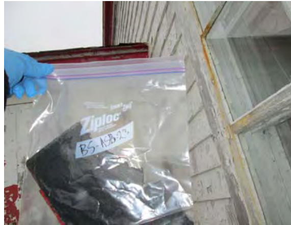
Photo 26: View of asphalt shingle with paper backing sample BS-ASB-23.
