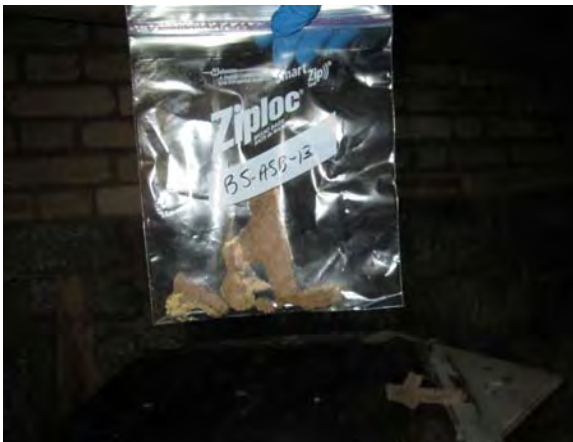
Photo 16: View of brick mortar sample BS-ASB-13.
