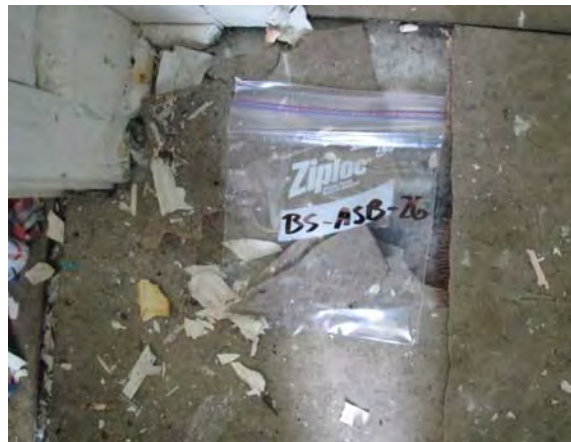
Photo 29: View of rolled flooring sample BS-ASB-26.
