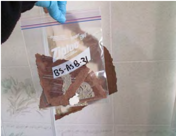
Photo 34: View of barker tile panel board sample BS-ASB-31.
