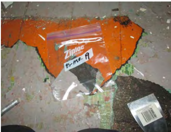
Photo 22: View of rolled flooring sample BS-ASB-19.
