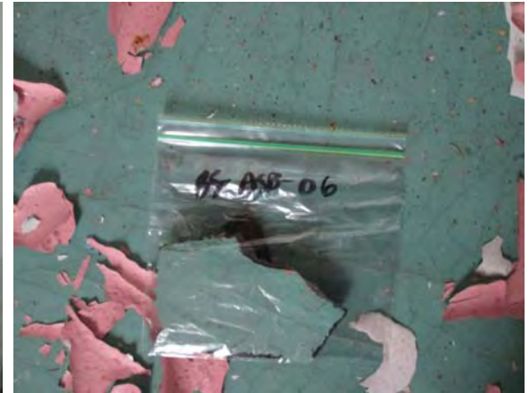
Photo 9: View of felt-type flooring sample BS-ASB-06.
