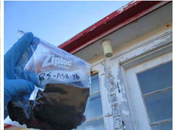
Photo 39: View of red/black asphalt shingle sample BS-ASB-36.
