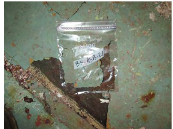
Photo 24: View of rolled flooring sample BS-ASB-21.
