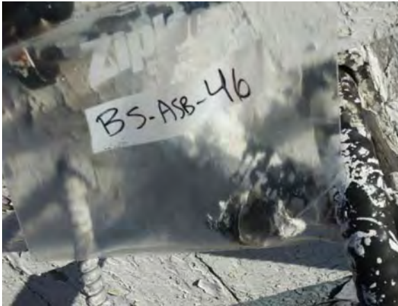
Photo 49: View of grey caulking sample BS-ASB-46.
