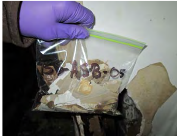
Photo 8: View of drywall joint compound sample BS-ASB-05.
