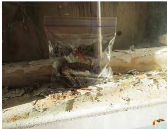
Photo 59: View of grey window caulking sample BS-ASB-56.
