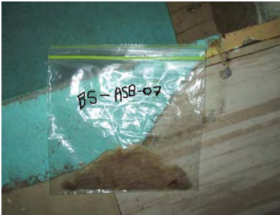
Photo 10: View of stair tread material sample BS-ASB-07.
