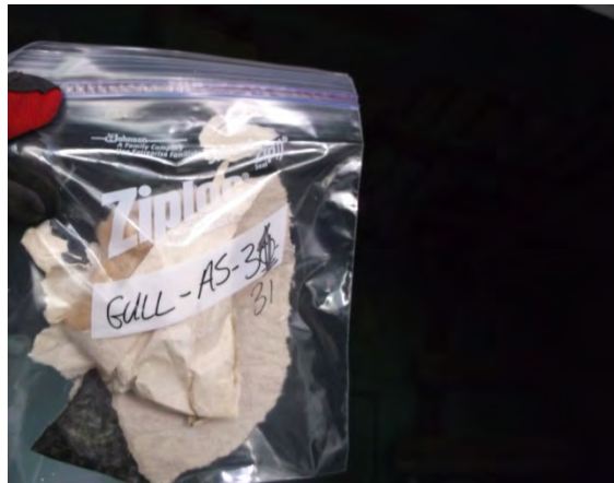
Photo 35: View of fiberglass insulation sample GULL-AS-31.
