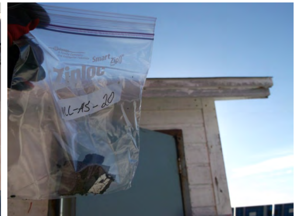
Photo 24: View of asphalt shingle with felt tar paper sample GULL-AS-20.
