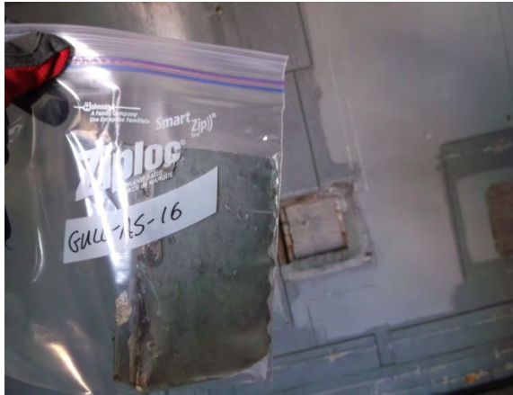
Photo 20: View of cement board (transite) sample GULL-AS-16.
