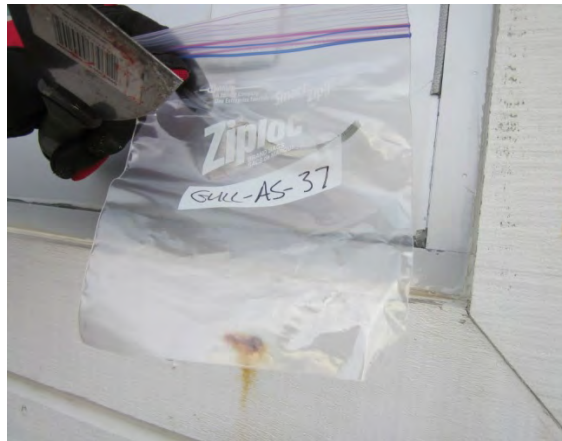
Photo 41: View of window caulking sample GULL-AS-37.
