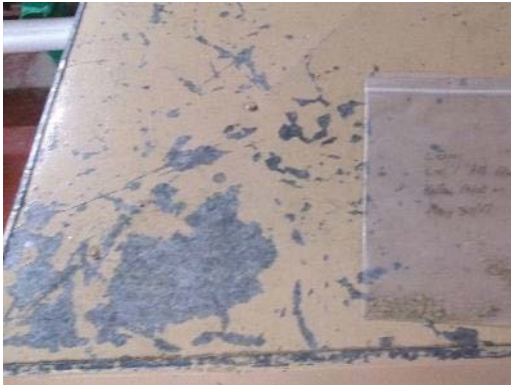
Lead-based "yellow" paint, Sample L0001.
