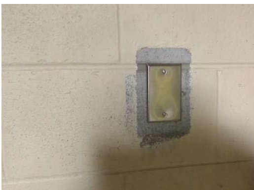
Lead-based "beige" wall paint, Sample L0005.
