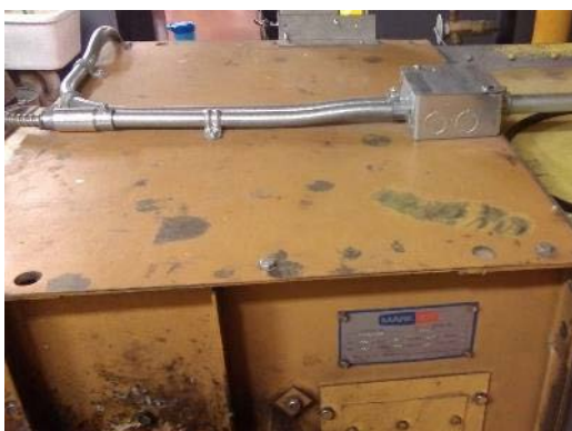
Lead-based "brown" paint, Sample L0003.
