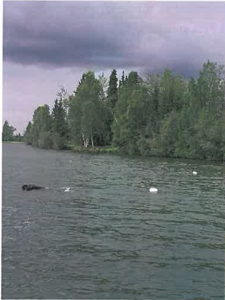
3 Coordinates marked with weighted line and floats, diver performing detailed search of shallow water.
