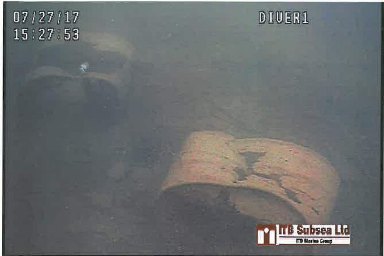
Photo 5: Multiple corroded barrels at 3m depth requiring removal.
