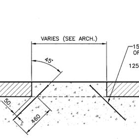
**DETAIL - TYPICAL ADD'L. REINFORCING AT DOOR OPENING**
