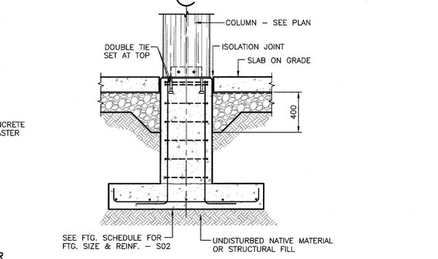
**DETAIL - TYPICAL INTERIOR FOOTING WITH PILASTER**
