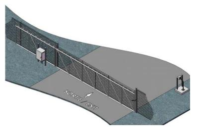
maximum opening/closing movement time is reached. The gate can be activated by push-buttons, remote control, keypad, card reader or any other similar device. Also, all security devices such as safety edges, loops and photoelectric cell can be connected to the control panel.
