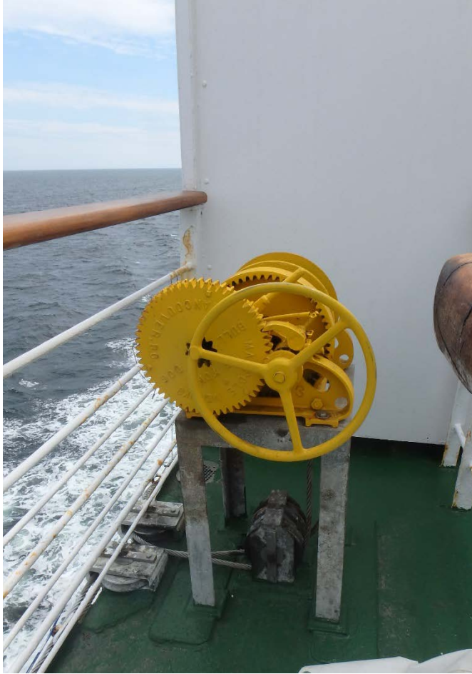
Figure 3: bowing winch with vertical & horizontal pulleys
