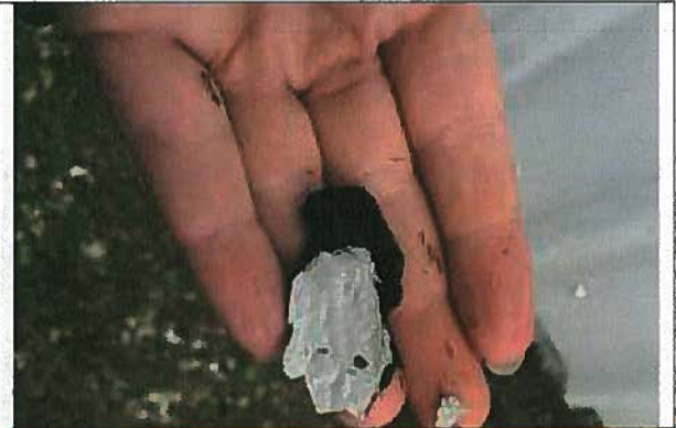
Sample: 27384-4 Location: West Exterior of the Building Description: Mastic Debris Hazardous Material: Chrysotile 8%
