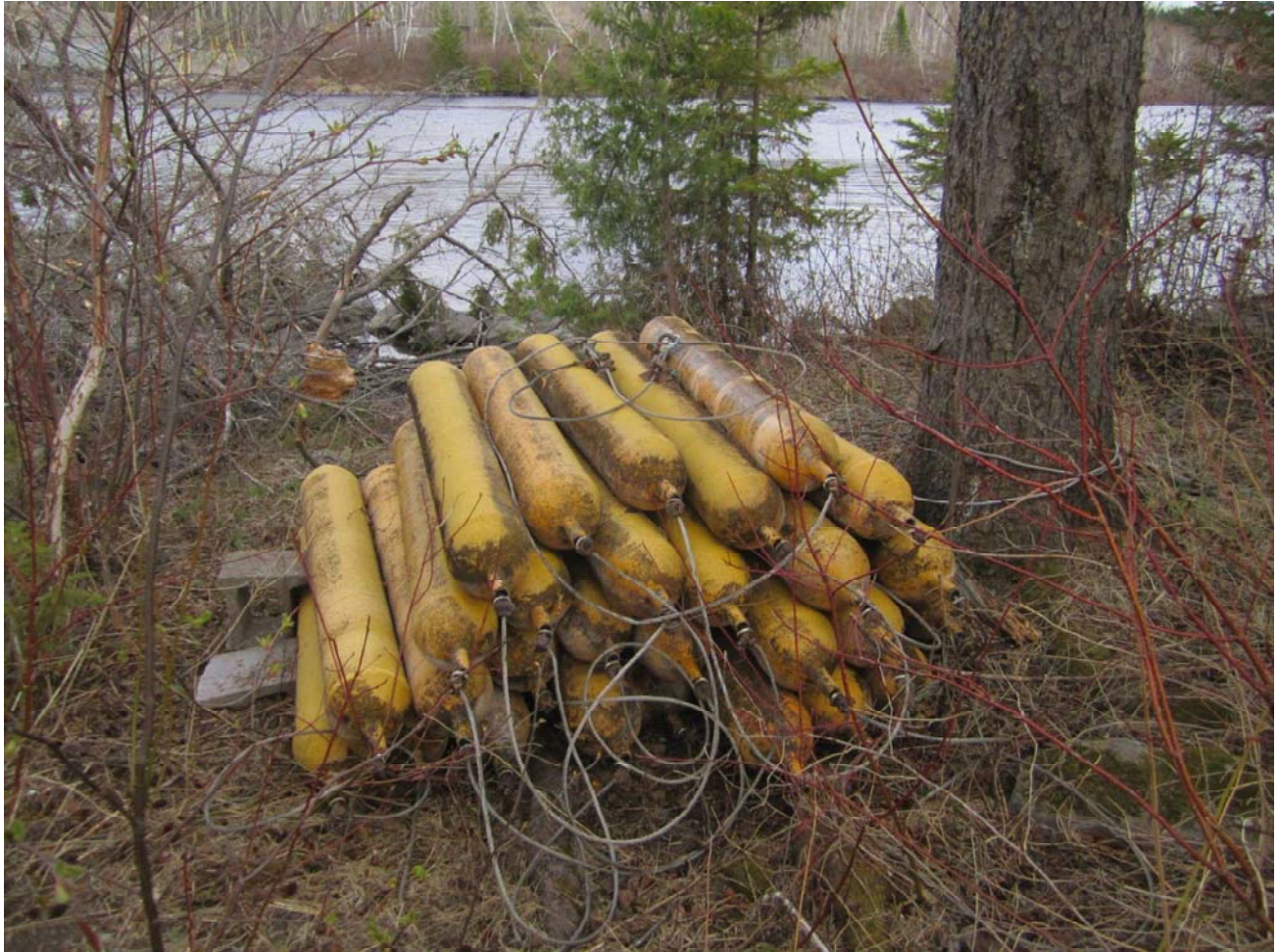
Figure 13: View of existing left shore (looking towards right shore). Existing booms shown in picture. Currently left shore anchor consists of wire secured around tree shown on the right.
