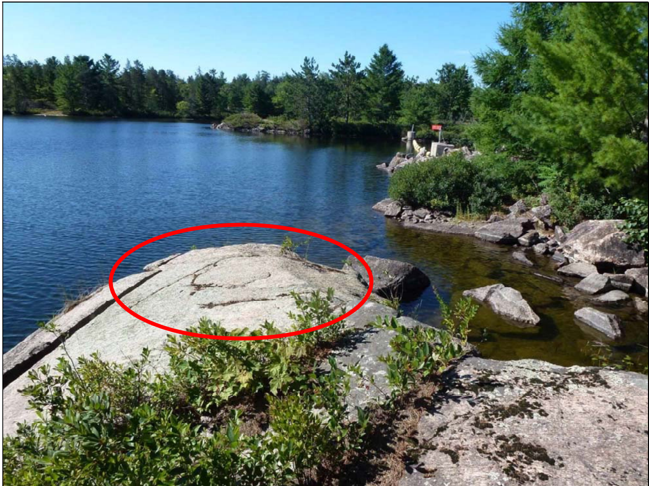
Figure 28: Portage Dam: area slightly upstream showing approximate anchor location of right anchor of new waterway barrier (rock in foreground). Existing waterway barrier anchors visible in upper right of photo. Water is flowing from left to right in this photograph. Proposed location of new right anchor circled in red.
