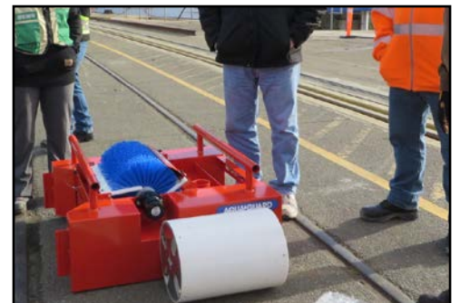
Spill response equipment: Skimmer.
