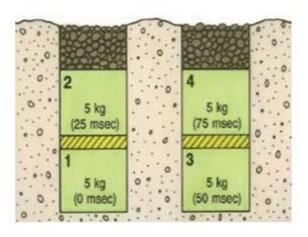
Per Fig. 1: 20 kg total weight of charge; 25 msecs delay between charges and blast holes and decking of charges within holes. (Fisheries and Oceans Canada, 2015)
