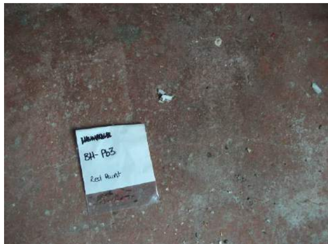
Photograph 29: Boat House Building – Lead-Based Red Floor Paint
