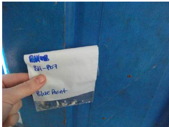
Photograph 30: Boat House Building – Lead-Based Blue Wall Paint
