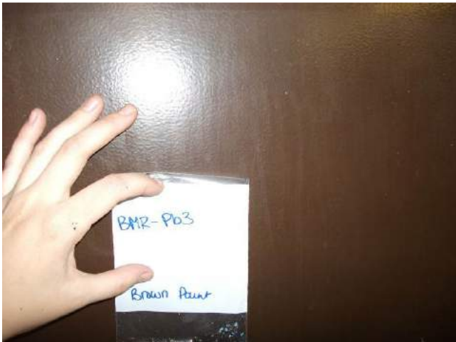
Photograph 35: Buoy Maintenance Building – Lead-Based Brown Exterior Paint
