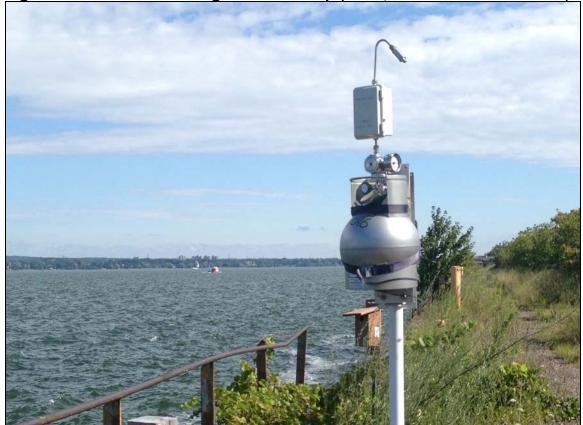
Figure 3 – EC Air Monitoring Station Set Up (timer, controller and canister)
